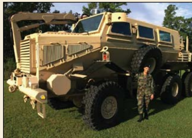
The Buffalo Armored Vehicle protects troops involved with clearing bombs and IEDs from roads in the combat zone
